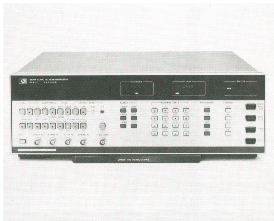
Fig. 1. Model 8170A Logic Pattern Generator produces long sequences of 8- or 16-bit parallel digital words as bus stimuli for functional tests of multichannel digital hardware. It operates at clock rates up to 2 MHz, internally or externally supplied.
